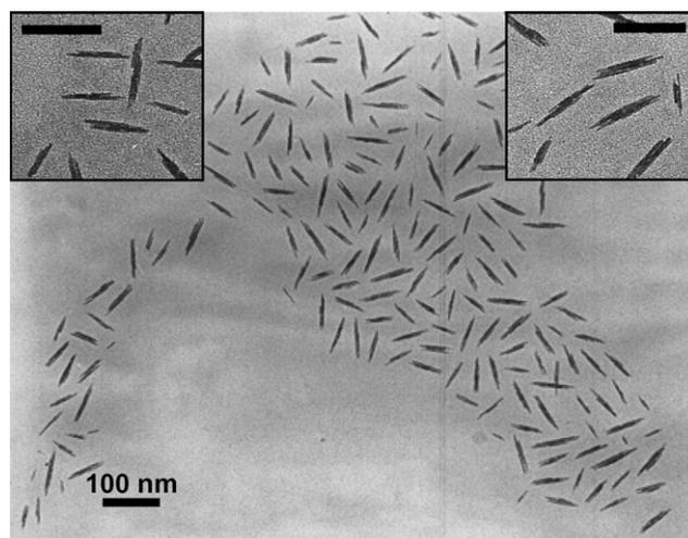
**Fig. 13** TEM image of lanthanum-based nanoparticles in the presence of PAA<sub>1000</sub>-b-PAM<sub>10000</sub> ( $R = 0.5$ ,  $h = 3$ ).
