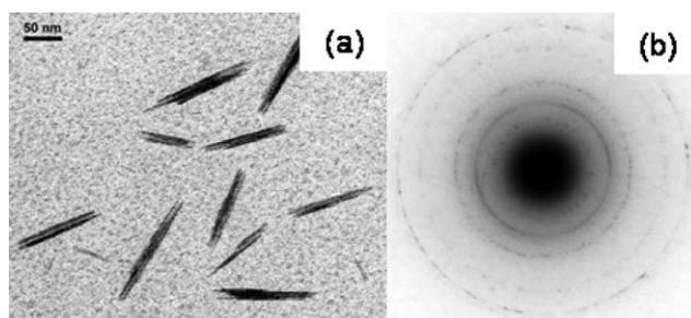
**Fig. 9** TEM image of lanthanum-based nanoparticles in the presence of  $\text{PAA}_{1000}\text{-b-PAM}_{10000}$  ( $R = 0.5, h = 3$ ) (a) and electron diffraction pattern of these colloids (b).
