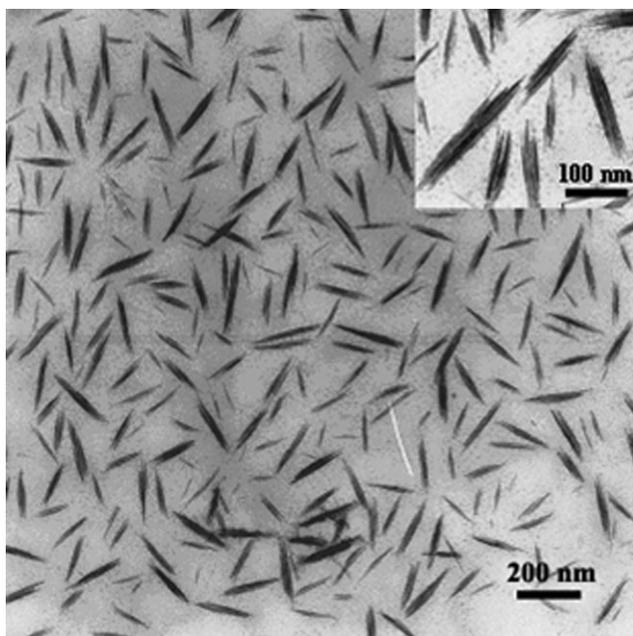
**Fig. 11** TEM image of lanthanum-based nanoparticles in the presence of PAA<sub>3000</sub>-b-PAM<sub>30000</sub> ( $R = 1$ ,  $h = 3$ ).
