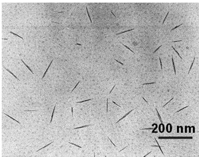
**Fig. 10** TEM image of lanthanum-based nanoparticles in the presence of PAA<sub>5000</sub>-b-PAM<sub>60000</sub> ( $R = 0.5$ ,  $h = 3$ ).
