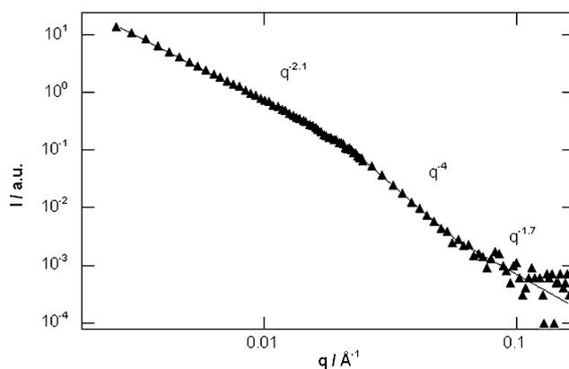
**Fig. 12** Neutron scattering intensity versus scattering vector  $q$  obtained from lanthanum based nanoparticles with PAA<sub>1000</sub>-b-PAM<sub>10000</sub> copolymer ( $R = 0.5$ ,  $h = 3$ ).
