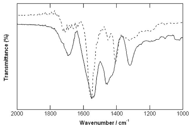
**Fig. 3** ATR-FTIR spectra of PAA (5100 g mol<sup>-1</sup>) homopolymer (dotted line) at pH 5.5 and a mixture La<sup>3+</sup> + PAA (5100 g mol<sup>-1</sup>) with a complexation ratio  $R = [\text{COO}]/[\text{La}] = 0.5$  (solid line).
