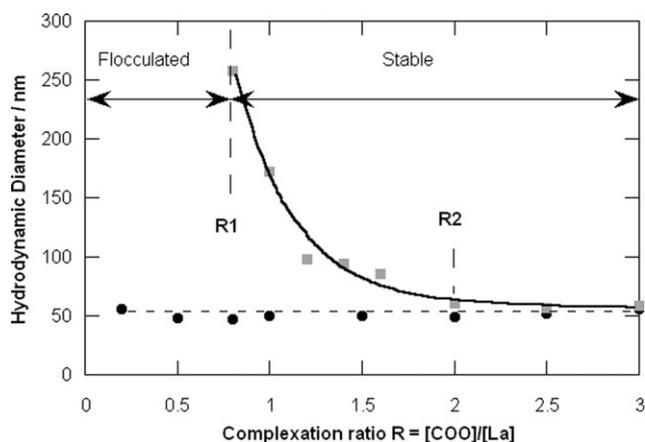
**Fig. 4** Influence of the complexation ratio on the size of the precursor aggregates (●) and of the mineralized particles (■) in the system  $\text{La}^{3+}$ -PAA<sub>5000</sub>-b-PAM<sub>30000</sub>. The curves in the graph serve as eye guides.
